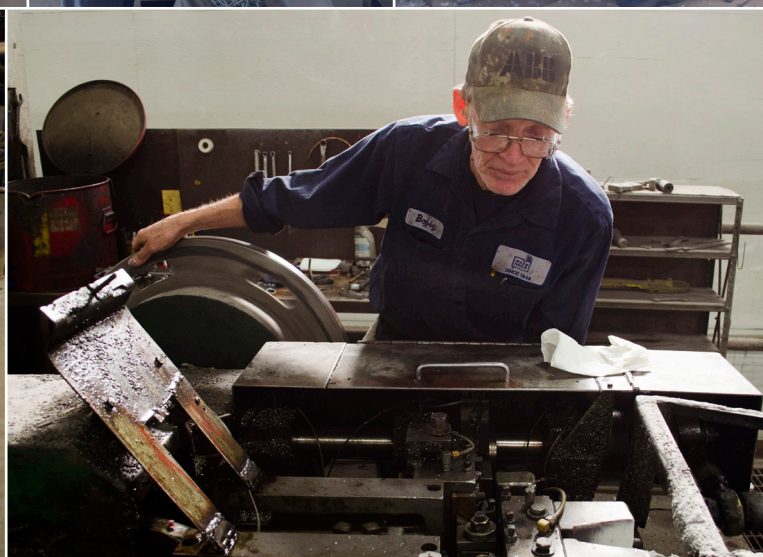
Bobby Lance fine tunes a nail machine that manufactures hundreds of nails every minute.
