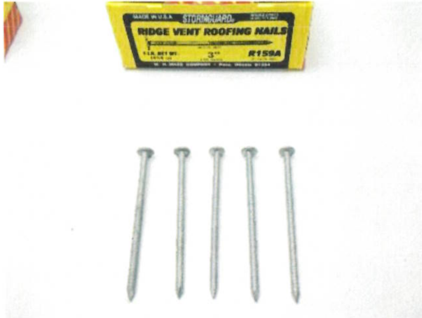
Photo No. 15 0.135" x 3" R159A Ring Shank Roofing Nails Prior to Salt Spray Exposure
