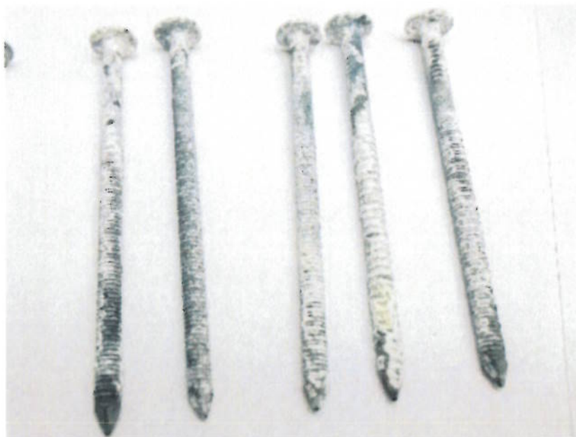
Photo No. 16 0.135" x 3" R159A Ring Shank Roofing Nails After Salt Spray Exposure
