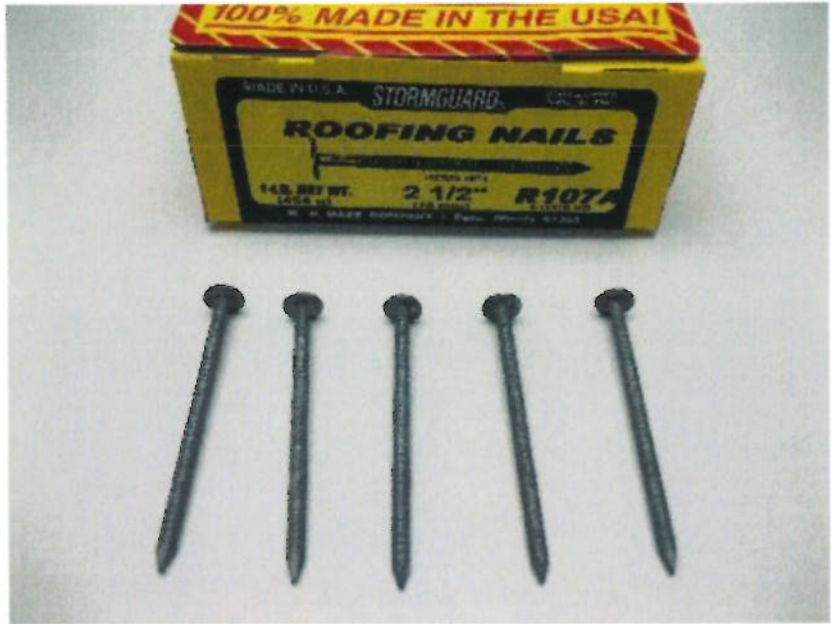
Photo No. 7 0.120" x 2-1/2" R107A Ring Shank Roofing Nails Prior to Salt Spray Exposure
