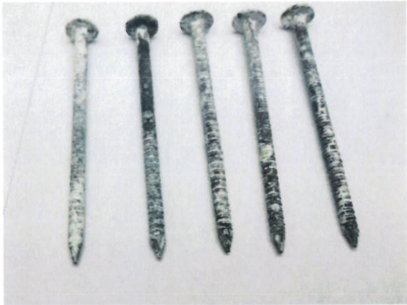
Photo No. 8 0.120" x 2-1/2" R107A Ring Shank Roofing Nails After Salt Spray Exposure
